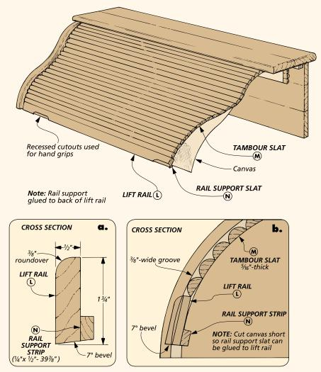
15a. Also, to match the profile of the slats, I used a  $3/_8$ " roundover bit to rout the top outside corner, refer to detail 'a' in drawing above.
