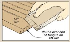
Lift rail. When a tambour won't slide freely, check the lift rail first. The sharp corners and edges can hang up in the groove. Use a sanding block to round over the end of the tongue.
