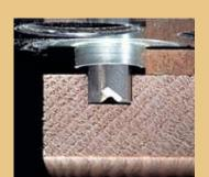
▲ A<sup>5</sup>/<sub>8</sub>"-dia. guide bushing installed in the router base rides against the template when routing the groove. Hold the bushing tight against the template for an exact copy of the profile.
