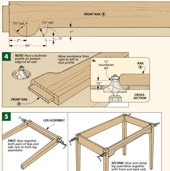
Then after cutting the top to finished size (24" x 43"), rout a bullnose profile on all four edges. Here again this required a 1/2" round-over bit, but this time I used a hand-held router.
