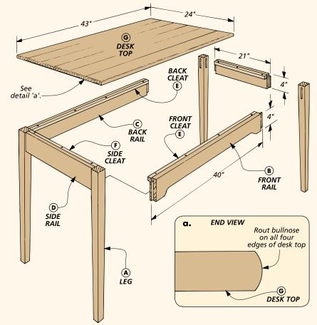
The **front rail (B)** and **back rail (C)** are 40" long, while the **side rails (D)** are only 21" long, see exploded view.
