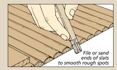
**Slats.** The slats can also hang up in the groove. Here again, round over the top and bottom ends. But because the groove is shallow, be sure to keep the radius small so it's not exposed.
