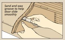
**Sand & Wax.** It's always a good idea to sand the groove lightly to remove any chatter marks left by the router. Then apply a coat of paste wax so the door will slide freely.
