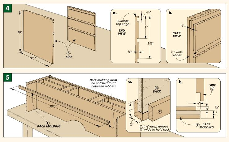
**MOLDING.** This back molding (F) is cut to fit between the rabbets in the sides, see Fig. 5. But this piece is  ${}^{3}/_{4}{}^{"}$  wide, while the rabbets are only  ${}^{1}/_{2}{}^{"}$  wide, so I had to notch the front corners to make it fit, see Fig. 5b.
