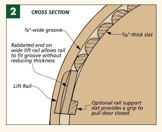
and the groove. You can't expect a  ${}^{3}/{8}^{"}$ -thick slat to slide very well in a  ${}^{3}/{8}^{"}$ -wide groove. The tambour door in the roll-top desk used  ${}^{5}/{16}^{"}$ -thick slats in a  ${}^{3}/{8}^{"}$  groove, see Fig. 2. This provided just enough clearance so the tambour door would slide smoothly but without rattling around when it moves.
