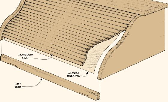
and pulled as the door is opened and closed. It's traditionally cut wider and thicker to make it stronger (like on the roll-top desk).
