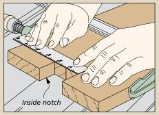
Check the Gap. Check your progress by clamping the boards together and measuring the gap created by the notches.
