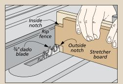
**Final Fit.** When the gap created by the notches is right on, you can complete the tenons by cutting the outside notches.
