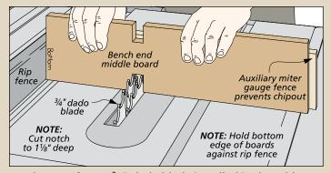
**Cutting Notches.** A  $\frac{3}{4}$ " dado blade installed in the table saw makes cutting the notches for the mortises an easy job. With the rip fence as a stop, just sneak up on the height.
