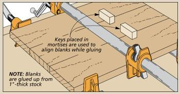
Assembling the End Blanks. The trick to assembling the end blanks is keeping the notches aligned. Waxed keys inserted before the clamps are tightened will solve the problem.
