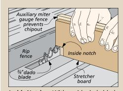
Inside Notches. With a wide dado blade on the saw and the fence set as a stop, sneak up on the height of the notches.
