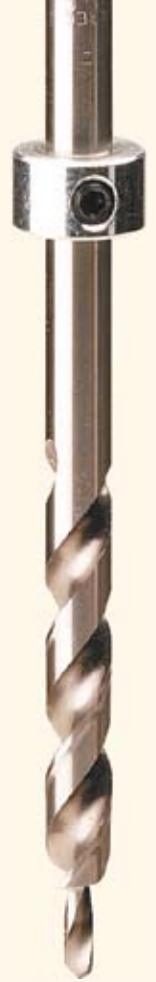
▲ Like two drill bits in one, the bit used for pocket holes drills the counter-bore and shank hole in one quick step. The stop collar ensures consistent results.
