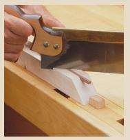
The workpiece is held by pressing it into a groove cut in the top of the miniature miter box. The end of the miter box is cut at an angle so it can be used for final trimming.
