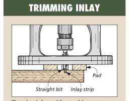
To trim inlay without chipout, tape a pair of pads onto the router base with some double-sided tape. Then adjust a straight bit so it's flush with the surface, and rout the inlay flush.
