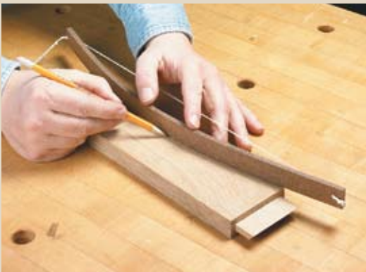
▲ A notched scrap of hardboard and a short length of string is all you need to lay out a smooth, consistent curve. A series of knots tied in one end of the string allows you to easily adjust the amount of "bow."
