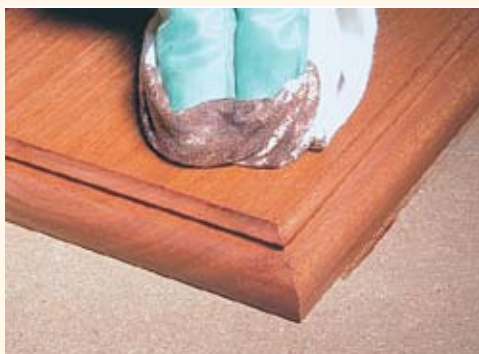
▲ After it's wiped off, you can see that the limited penetration of a gel stain means the end grain is the same color as the face grain.
