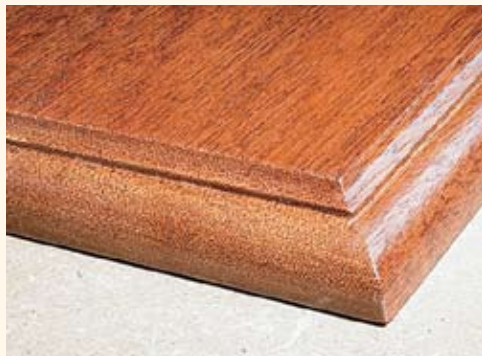
▲ One solution to evening out the end grain is to sand it finer than the rest of the board. Here, I sanded the end grain to 600-grit.
