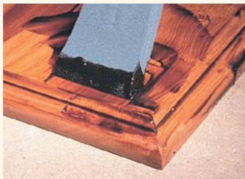
▲ A gel stain is just a thick stain. Its thickness limits the amount it penetrates, so I usually work it into the pores with a brush.
