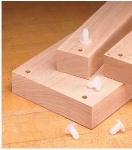
▲ Plastic "stem bumper glides" are added to the front of all the lower drawer supports (and top, back corners of the drawers) so the drawers slide in and out of the case smoothly.
