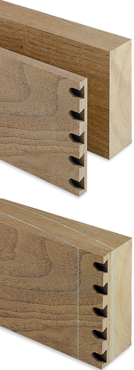
▲ The dovetails are routed first (top). Then add a thick blank (bottom), and cut the front to shape.
