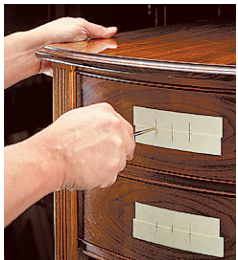
▲ When laying out the pilot holes for mounting the pulls, I protected the finish with strips of masking tape.
