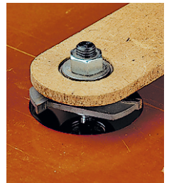
▲ To cut a \frac{1}{4} "-deep groove on the drawer front, I used a slot cutter bit and a shop-made rub arm, as described in Shop Notes on page 13.
