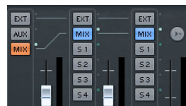
Control Room Mixer channels with active Signal Presence indicators
