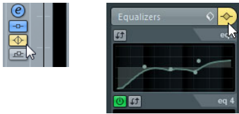
Left: EQ bypass in the Mixer; Right: EQ bypass in the Channel Settings window or the Inspector
