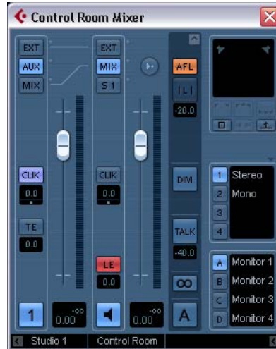
A Studio channel in the Control Room Mixer with its input set to Aux.
