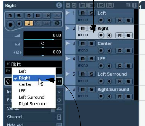
Step 2 - Open the “Input Routing” pop-up menu and select the input for the track.
