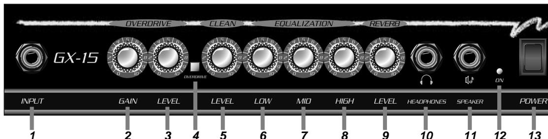
**1: INPUT:** Use this 1/4" jack to connect your guitar to the amplifier by means of a shielded instrument cable.
