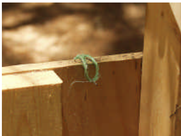
Figure A-2. A rear view of the top of a box baler showing the nail used to hold the baling string in place as pine straw is loaded into the baler.
