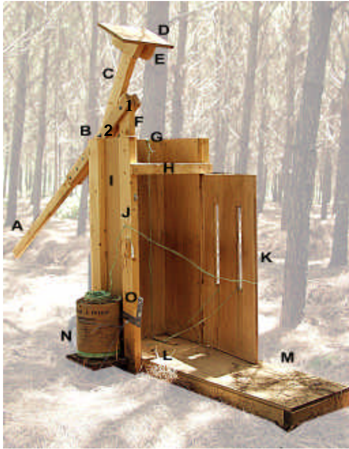
Figure A-1. Illustration of a typical, easy to construct hand-powered, box baler showing the main components.
