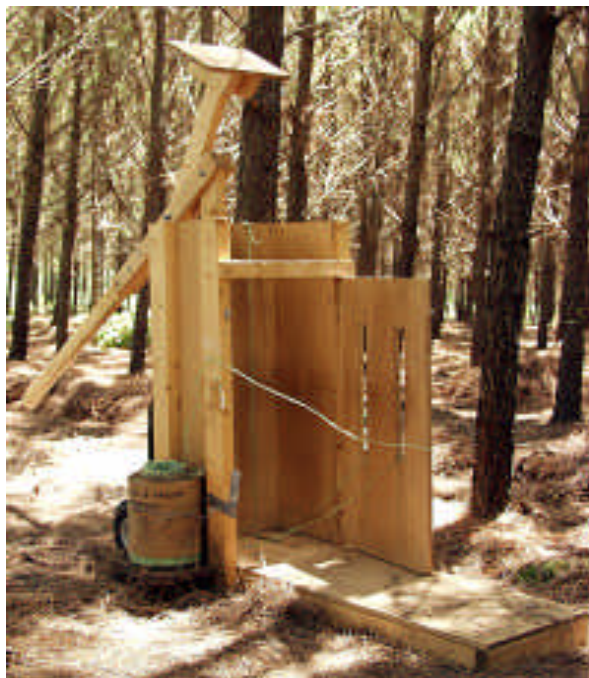
Figure 4. Pine straw can be baled with a simple hand-powered box baler.
