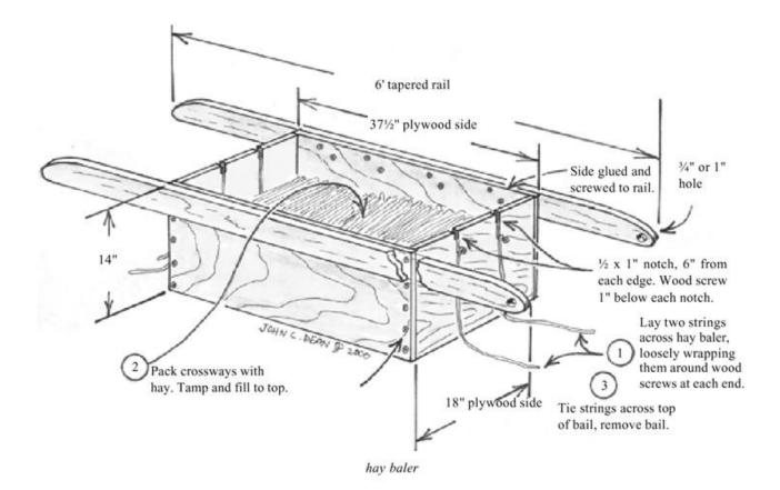
The entire "baler" can be put together in just a couple of hours, using only a single  $4 \times 8$  sheet of 3/4" plywood, a couple of six-foot 2x4s, some 1-1/2" wood screws, and a tube of construction adhesive. If you keep it painted or varnished for protection from the elements, it should hold up to at least a lifetime of use.
