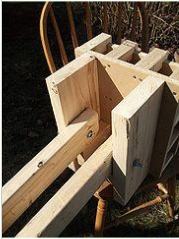
Fig 21: Completed Piston with Bolts
