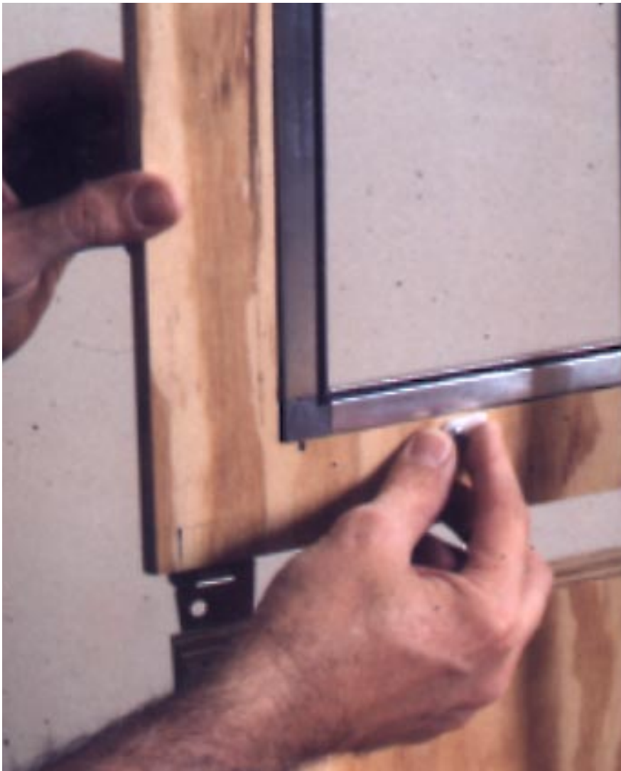
Nylon turn buttons hold the interchangeable inserts in the lid. You also can glaze the lid directly with a piece of clear acrylic sheet.
