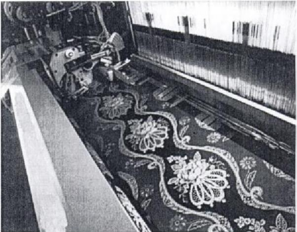
FIGURE 6.43 Jacquard shedding offers endless design pattern possibilities.
