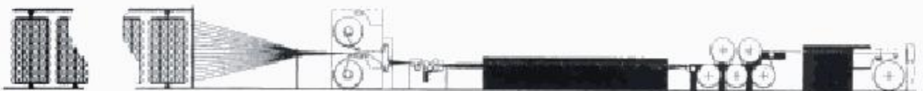
FIGURE 4.78 Sizing yarns from package creels and warp beams (courtesy of Benninger).
