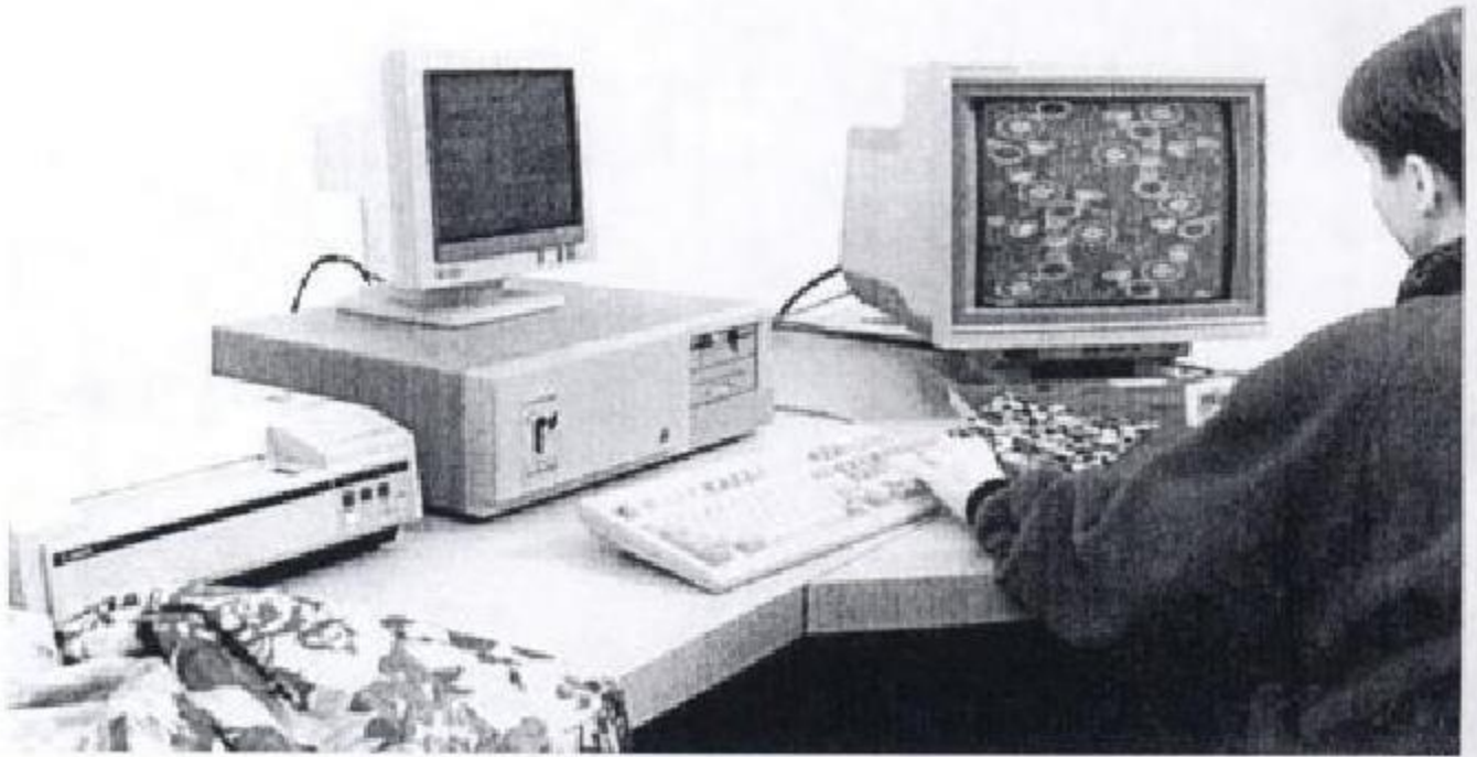
FIGURE 14.20 CAD of a jacquard design (courtesy of Staubli).
