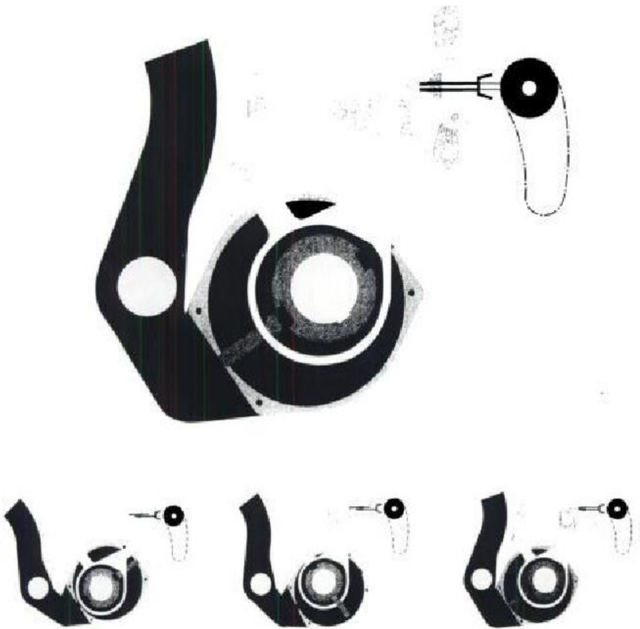
FIGURE 6.29 Functional principle of positive rotary dobby with pattern card control (courtesy of Staubli).
