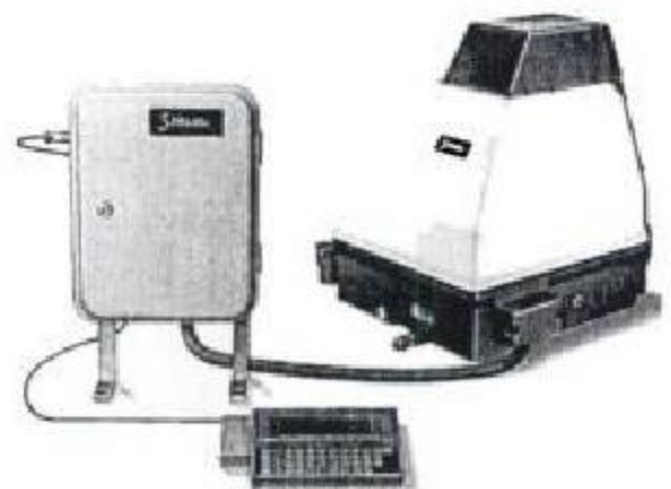
FIGURE 6.15 Computer programming system for dobbie weaving (courtesy of Staubli).
