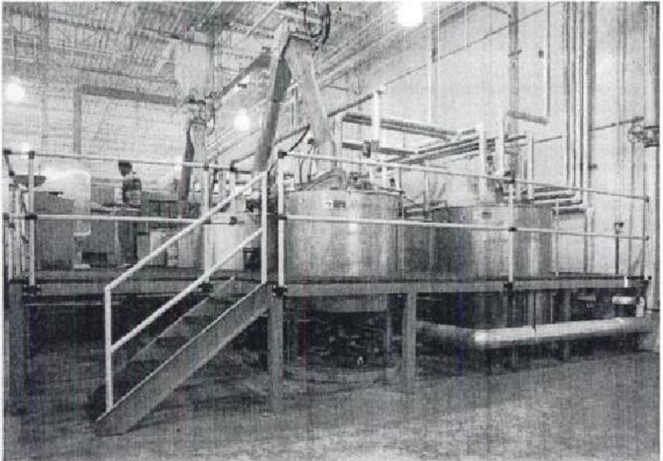
FIGURE 4.74 Rotor-cooker and size preparation units (courtesy of West Point Foundry and Machine Company).
